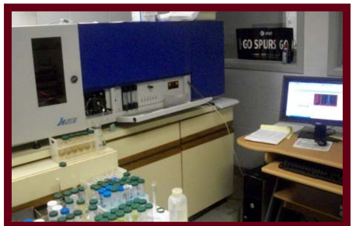
A mass spectrometer used to analyze metals and inorganic compounds at Alamo Analytical Laboratories
