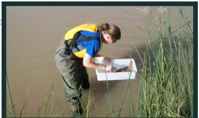
USIBWC CRP collects sediment to test for organics at Station 13272 in El Paso, Sept. 2010
