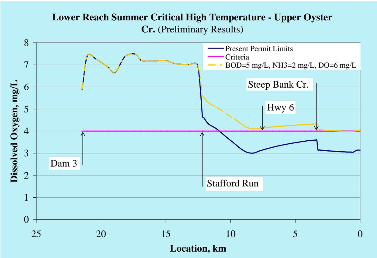
Figure 4. Example QUAL2K application on Upper Oyster Creek evaluating increased permit limits on domestic wastewater treatment plant discharges
