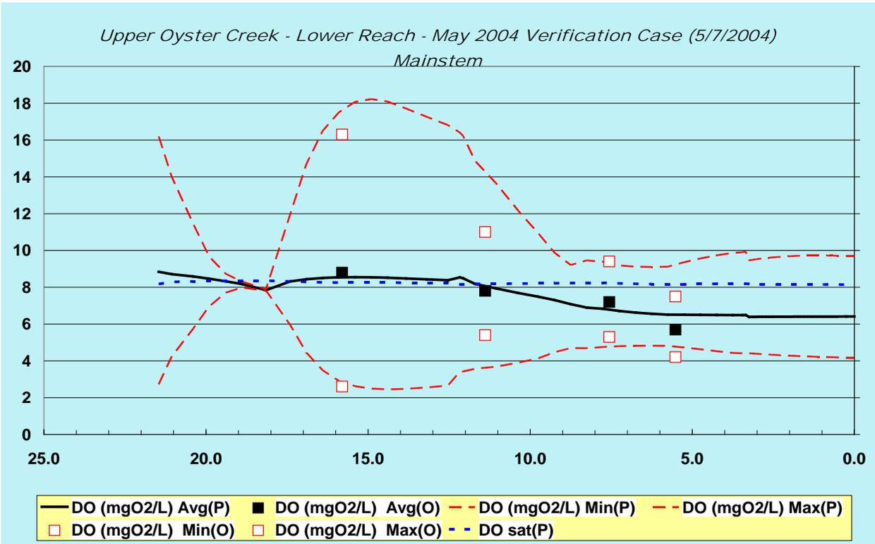
Figure 3. Example dissolved oxygen calibration / validation for Upper Oyster Creek
