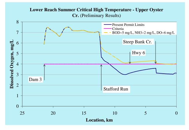
Figure 4.Example QUAL2K application on Upper Oyster Creek evaluating increased permit limits on domestic<br/>wastewater treatment plant discharges
