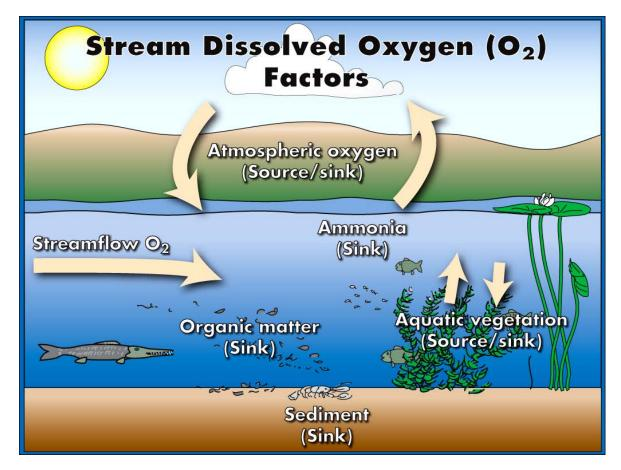
Figure 2. Schematic of processes affecting DO levels which are modeled in QUAL2K
