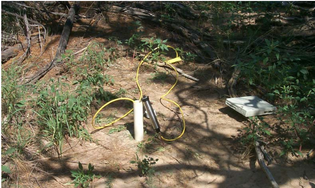
Figure 4. Photo of groundwater monitoring well
