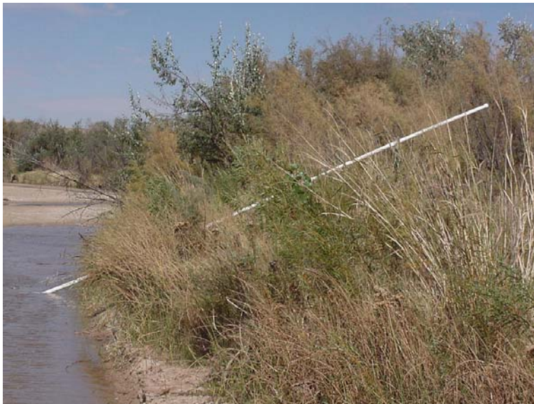
Fig. 3. River well installed at Canadian location.
