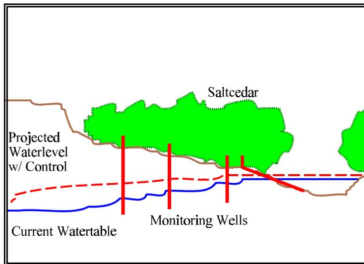
**Figure 1.** Schematic depicting the location of groundwater monitoring wells, river level monitoring well, and projected watertable/level following control of saltcedar. The difference between water levels before and following treatment will allow calculation of the total volume of water saved, excluding soil component.
