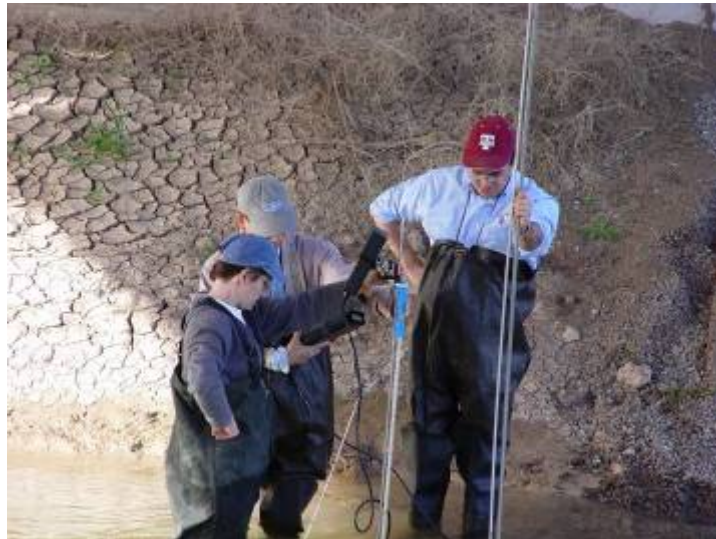
River flow measurement using sonic FlowTrac
