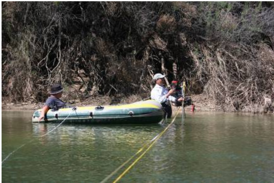
River flow measurement at Pecos River study site
