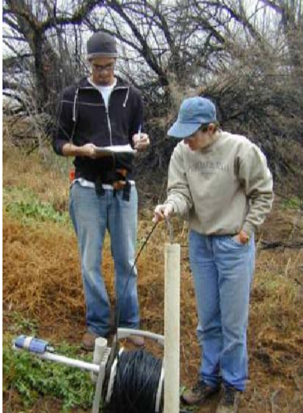
Recording water levels in a monitoring well
