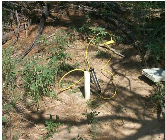
Pressure sensitive data loggers used to calculate water loss
