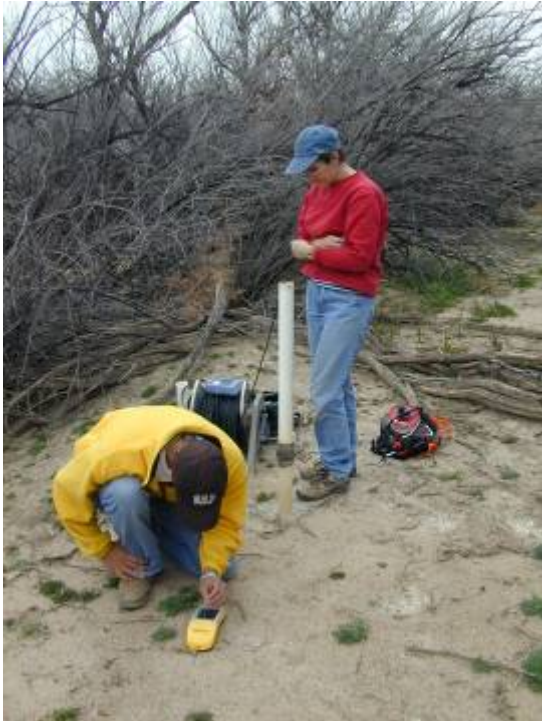
Pressure sensitive data loggers used to calculate water loss
