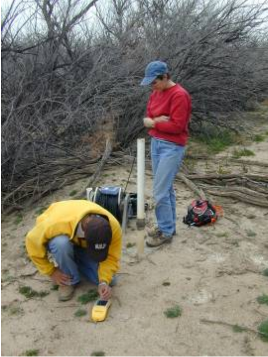
Collecting water levels and water quality data from a monitoring well
